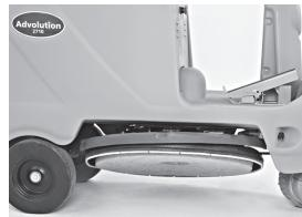
Mid-mounted, burnishing head tilts up for access to change burnishing pads quickly and easily.
